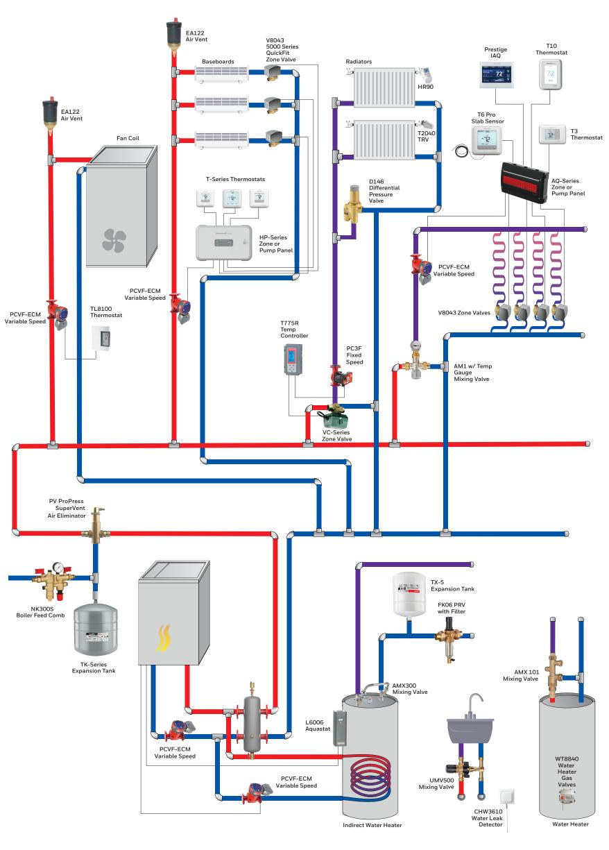
Not a typical system. Illustration for reference purposes only. Note: This is only a concept drawing. Designer must design injection and multi-zone systems from the ground up to ensure proper working of the system and compliance with code requirements.
