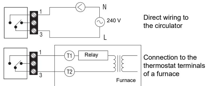
**For a 3-wire connection:** observe the polarity
