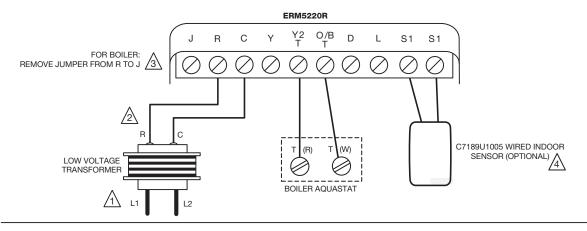
WIRING AT THERMOSTAT IF CUSTOMER ALSO HAS FORCED AIR COOLING OR A HYDRO-AIR APPLICATION (NOT REQUIRED ON HEAT ONLY APPLICATIONS)
