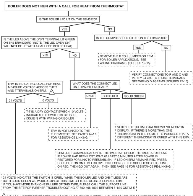
YOU CANNOT TEST THESE TERMINALS WITH A CONTINUITY METER. WHEN WIRES ARE NOT CONNECTED TO THESE TERMINALS, THERE WILL BE INFINITE RESISTANCE ACROSS THE TERMINALS WHETHER THE DRY CONTACT SWITCH IN THE ERM IS OPEN OR CLOSED. ONLY TEST WITH THE WIRES CONNECTED.
