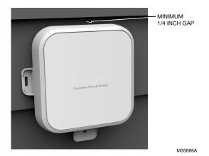
Fig. 7. If mounting on lap siding, allow space for the cover to be removed.
