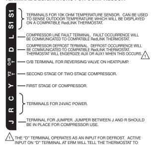
Fig. 4. Terminal Designations for Compressor.
