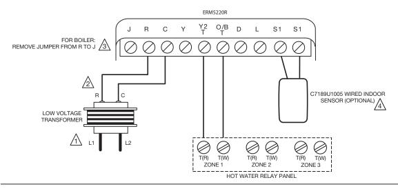
WIRING AT THERMOSTAT IF CUSTOMER ALSO HAS FORCED AIR COOLING OR A HYDRO-AIR APPLICATION (NOT REQUIRED ON HEAT ONLY APPLICATIONS)
