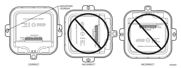
Fig. 6. Mounting orientation.
