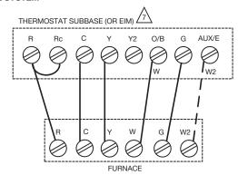
WIRE TRANSFORMER PRIMARY TO APPROPRIATE 120, 208, OR 240 VOLTAGE POWER SUPPLY AT OUTDOOR UNIT. TRANSFORMER NOT NECESSARY IF THERE ARE TWO WIRES AVAILABLE FROM R AND C ON INDOOR UNIT TO R AND C ON ERM. FOLLOW TRANSFORMER INSTALL GUIDE FOR WIRING OF TRANSFORMER PRIMARY.
