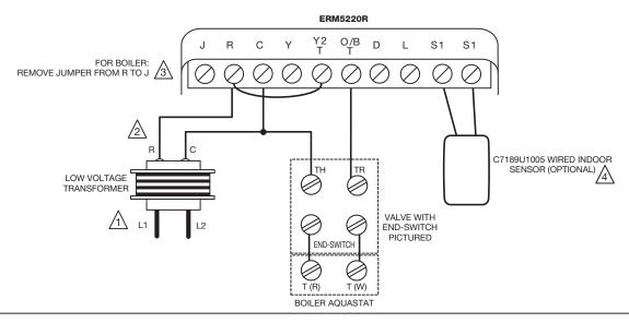
WIRING AT THERMOSTAT IF CUSTOMER ALSO HAS FORCED AIR COOLING OR A HYDRO-AIR APPLICATION (NOT REQUIRED ON HEAT ONLY APPLICATIONS)
