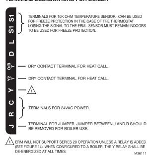
Fig. 5. Terminal Designations for Boiler.
