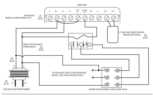
WIRING AT THERMOSTAT IF CUSTOMER ALSO HAS FORCED AIR COOLING
