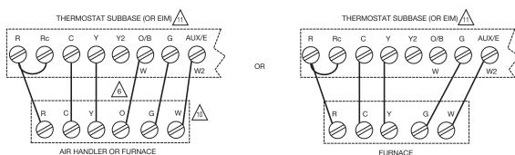
WIRE TRANSFORMER PRIMARY TO APPROPRIATE 120, 208, OR 240 VOLTAGE POWER SUPPLY AT OUTDOOR UNIT. TRANSFORMER NOT NECESSARY IF THERE ARE TWO WIRES AVAILABLE FROM R AND C ON INDOOR UNIT TO R AND C ON ERM. FOLLOW TRANSFORMER INSTALL GUIDE FOR WIRING OF TRANSFORMER PRIMARY.
