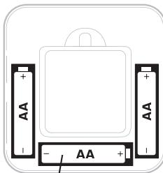
Insert 3 AA batteries for primary or backup power. Match the polarity of the batteries with the + / - marks inside the battery compartment.
