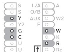
Note: Not all terminals may be used, depending on the system type that is being wired. The most commonly used terminals are shaded.
