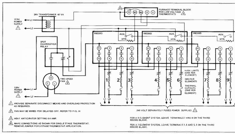
FIG. 10—WIRING SCHEMATIC FOR A 9 ELEMENT 240/120 VOLT SYSTEM—ISOLATED FAN.
