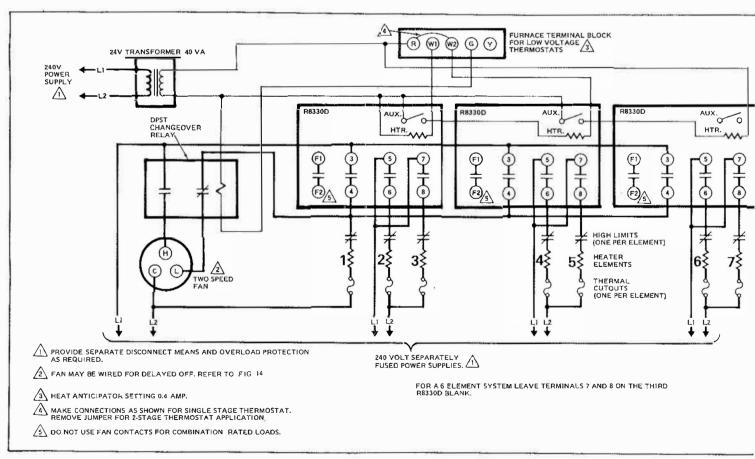
FIG. 13—WIRING SCHEMATIC FOR UP TO 7 ELEMENT 240 VOLT SYSTEM—COMBINATION RATED.
