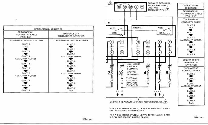
FIG. 9-WIRING SCHEMATIC FOR UP TO 6 ELEMENT 240/120 VOLT SYSTEM-ISOLATED FAN.
