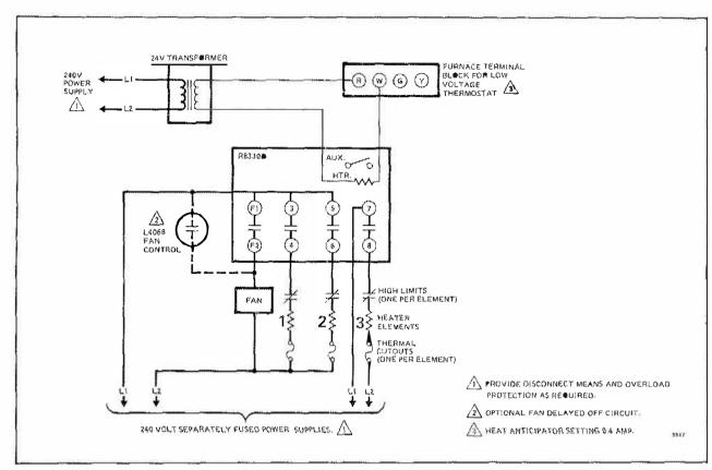
FIG. 14-SINGLE SPEED FAN WIRING.
