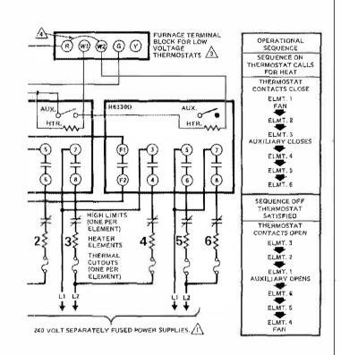
FOR A S ELEMENT SYSTEM, LEAVE TERMINALS ? AND 8 ON THE SECOND R8330D BLANK.
