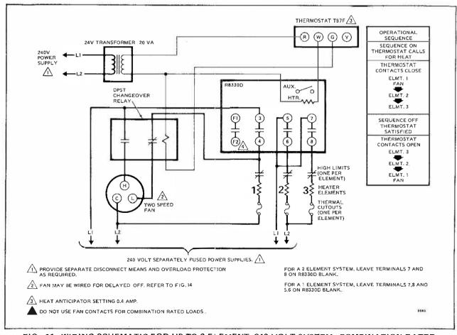
FIG. 11-WIRING SCHEMATIC FOR UP TO 3 ELEMENT 240 VOLT SYSTEM-COMBINATION RATED.
