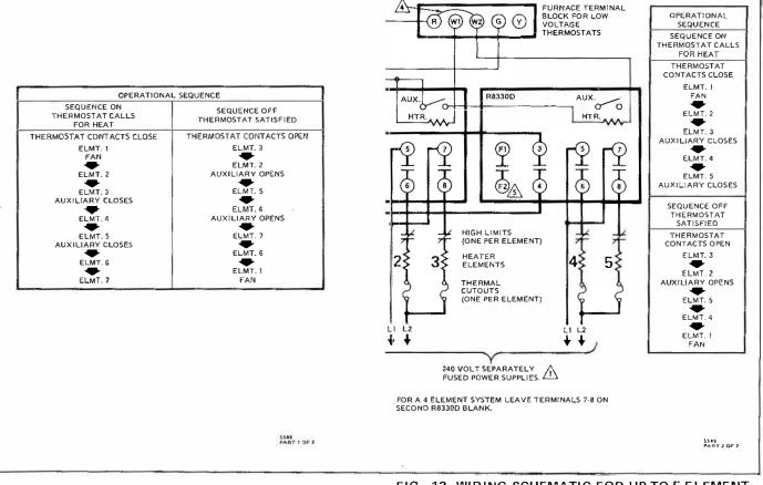
FIG. 12-WIRING SCHEMATIC FOR UP TO 5 ELEMENT 240 VOLT SYSTEM-COMBINATION RATED.
