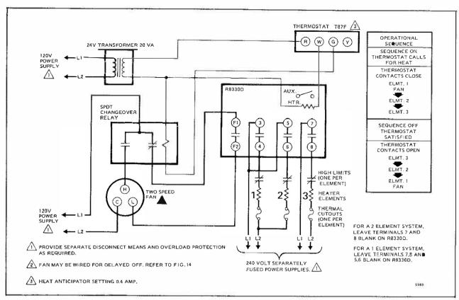
FIG. 8-WIRING SCHEMATIC FOR UP TO 3 ELEMENT 240/120 VOLT SYSTEM-ISOLATED FAN.
