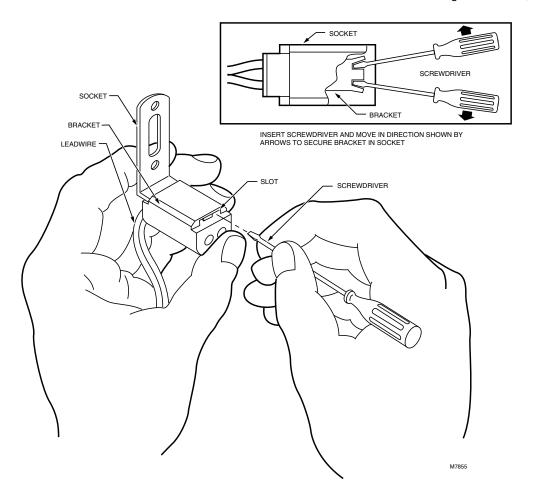
While holding the mounting bracket in the slot, insert the screwdriver in the other end of the slot (Fig. 4). Bend the screwdriver, first to the left and then to the right, to crimp the end of the mounting bracket and hold it in position.
