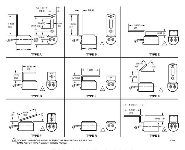
Fig. 1. Mounting bracket dimensions in in. (mm).
