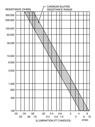
Fig. 7. Light response tolerance for C554A cad cell.
