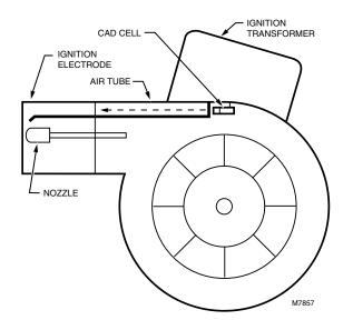
Fig. 2. Cad cell location.
