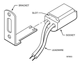
Fig. 3. Insert mounting bracket into socket slot.
