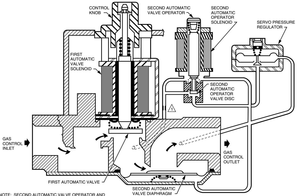
NOTE: SECOND AUTOMATIC VALVE OPERATOR AND SERVO PRESSURE REGULATOR SHOWN OUTSIDE GAS CONTROL FOR EASE IN TRACING GAS FLOW.
