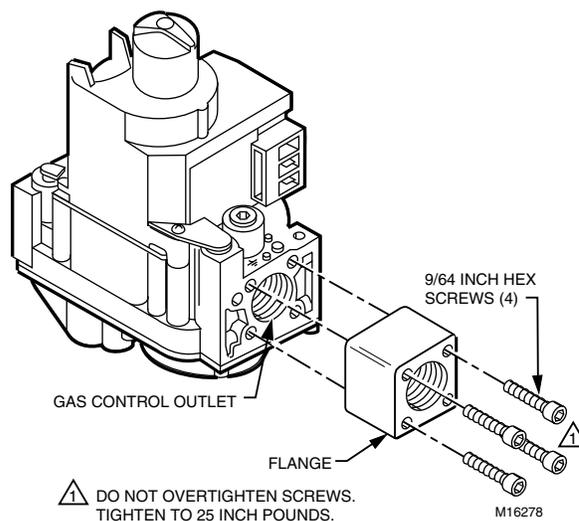
space limitations. This problem can be resolved for most installations by using an adapter. The adapter is installed on the end of the supply pipe in place of the gas control, following the same precautions and instructions that are used for installing the gas control. After the adapter is installed, the gas control is attached to the adapter as outlined above. Note that using an adapter increases the overall length of the gas control.
