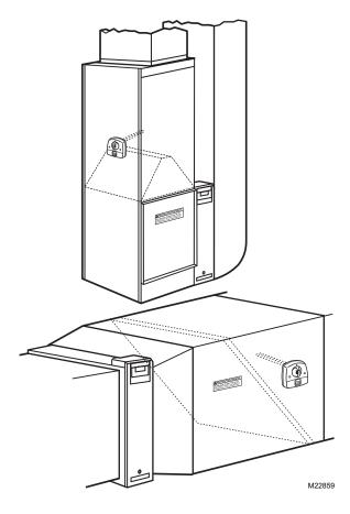
Fig. 2. Typical Surface Treatment installations.
