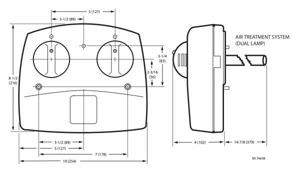
Fig. 3. Ultraviolet System dimensions in in. (mm).
