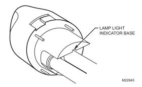
Fig. 12. Wipe lamp light indicator base.
