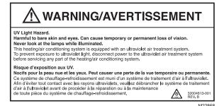
Fig. 8. HVAC maintenance UV safety label.
