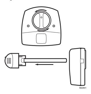
Fig. 10. Remove lamp bulb.
