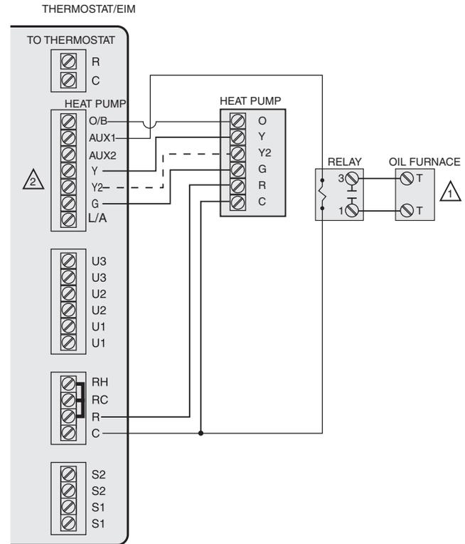
**Fig. 320. Heat pump with oil forced air backup.**
