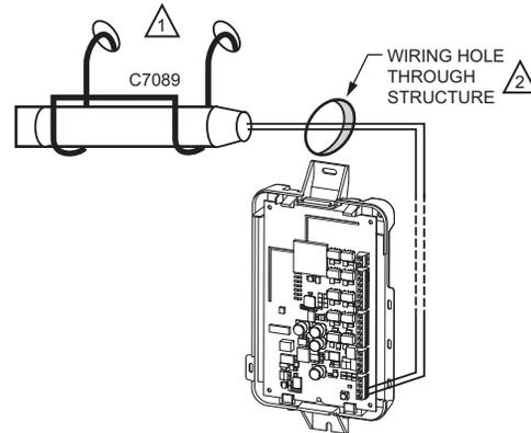
1 USE APPROPRIATE MOUNTING MEANS FOR THE TYPE OF STRUCTURE.
