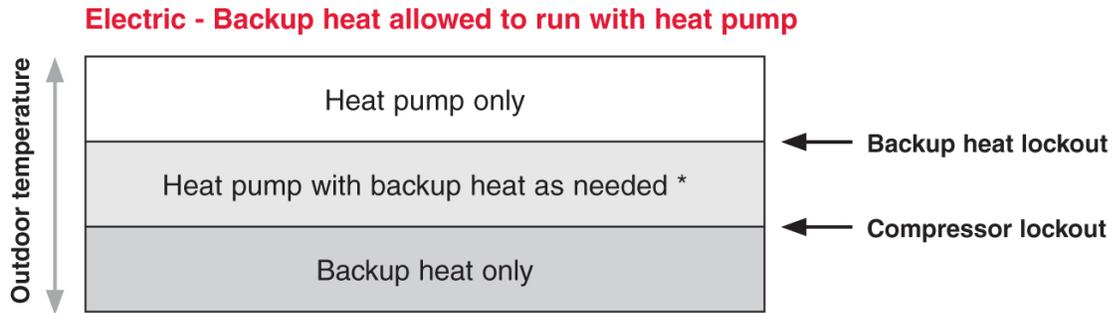
\* No backup heat unless indoor temperature drops to selected Backup Heat Droop setting, or Backup Heat Upstage Timer expires. **Heat pump stays ON when backup heat turns on.**
