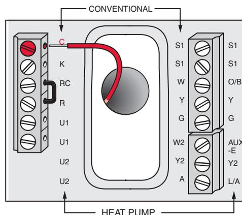
**Fig. 18. Connecting C wire to terminal block.**
