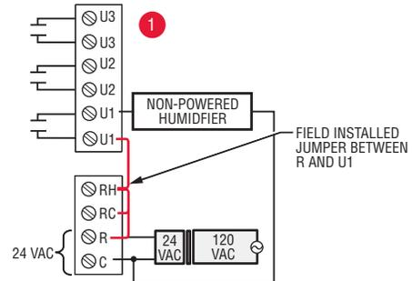
**Fig. 335. Typical hookup of non-powered humidifier.**
