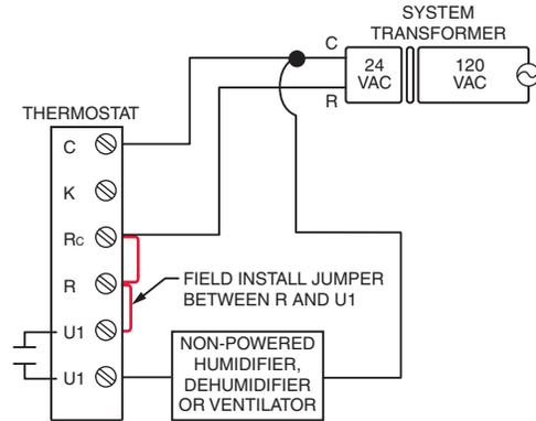
**Fig. 330. Wiring a non-powered humidifier, dehumidifier, or ventilator.**
