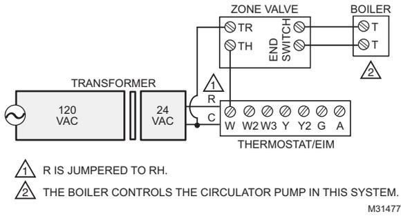
**Fig. 317. 2-Wire Zone Valve with end switch.**
