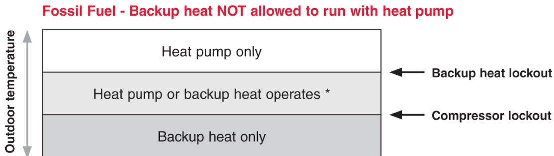
\* No backup heat unless indoor temperature drops to selected Backup Heat Droop setting, or Backup Heat Upstage Timer expires. **Heat pump turns OFF when backup heat turns on.**
