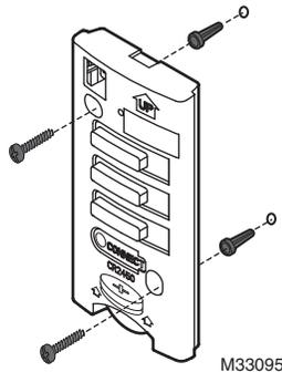
**Fig. 77. Mounting Entry/Exit Remote or Vent Boost Remote.**
