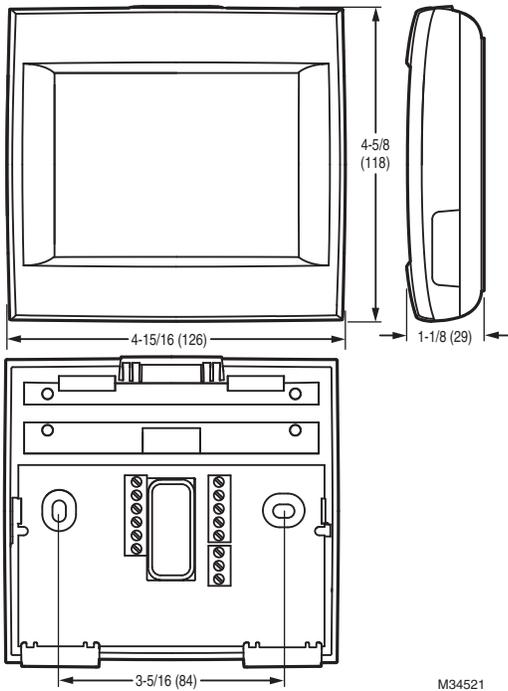
**Fig. 1. Dimensions of thermostat in in. (mm).**
