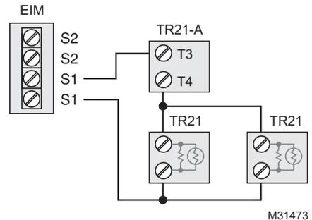
**Fig. 347. Wiring 2 TR21 sensors and 1 TR21-A sensor.**
