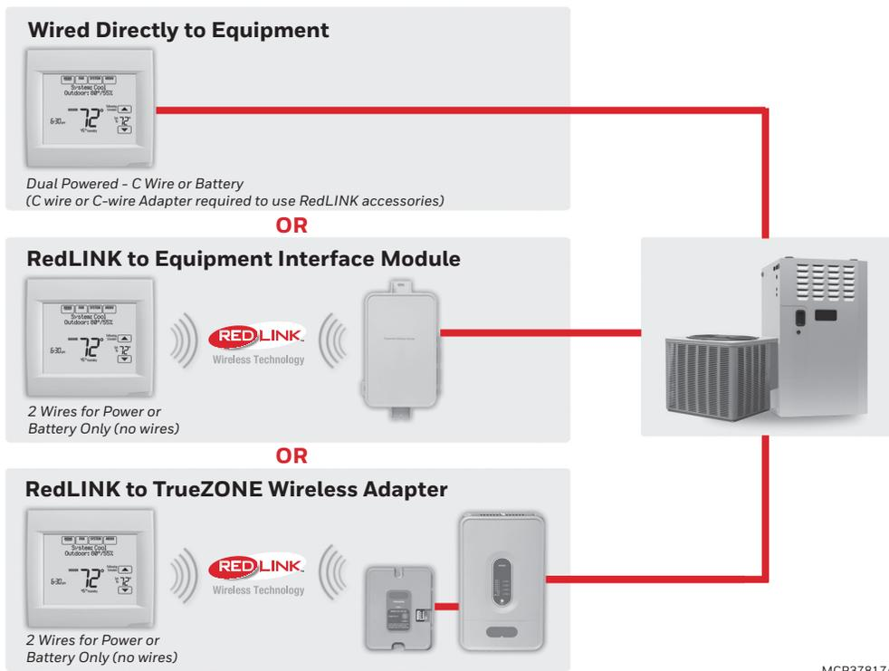
Fig. 5. VisionPRO® 8000 with RedLINK® 2.0 installation options.
