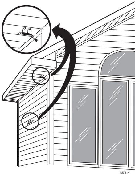
**Fig. 73. Typical locations for C7089U1006 Outdoor Sensor.**
