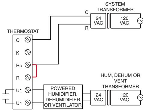
**Fig. 328. Wiring a powered humidifier, dehumidifier, or ventilator.**
