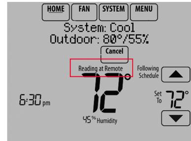
**Fig. 303. Reading temperature at the Portable Comfort Control.**
