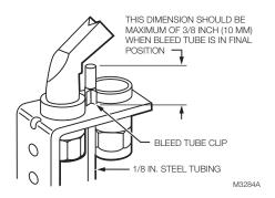
Fig. 6. Install bleed gas tubing.
