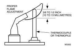
Fig. 8. Thermocouple/thermopile tip must be in pilot flame.
