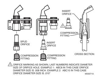
Fig. 7. Changing spud and insert orifices.
