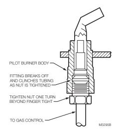
Fig. 3. Always use new compression fitting.
