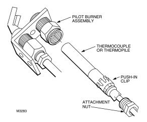
Fig. 4. Installing thermocouple or thermopile.
