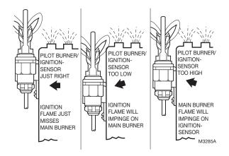
Fig. 2. Location of pilot burner.
