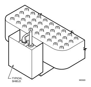
Fig. 9. Proper shielding of pilot flame.
