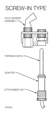
Fig. 5. Installing Q390 Thermocouple.
