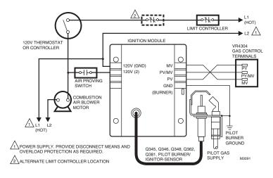
Fig. 7. VR4304 wiring connections in intermittent ignition system.
