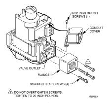
Fig. 1. Install flange to gas control.
