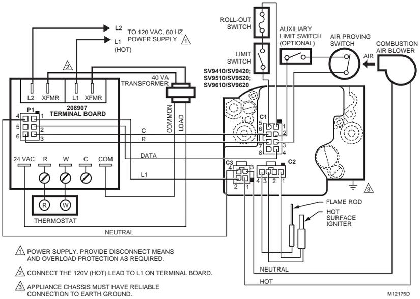
Fig. 8. SV9410/SV9420; SV9510/SV9520; SV9610/SV9620 typical wiring connection with 208907 Terminal Board.
