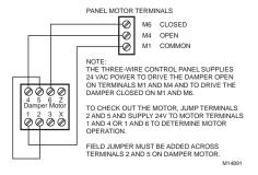
Fig. 2. Wiring a single damper from a three-wire control panel.
