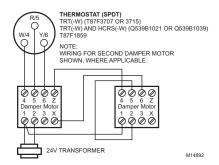
Fig. 3. Wiring two dampers in tandem from a threewire thermostat.
