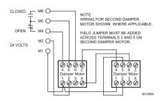
Fig. 5. Wiring five-wire control panel with two dampers to one zone.
