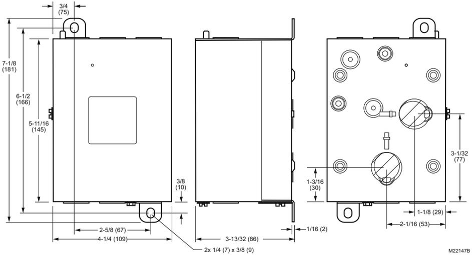
Fig. 1. L7103 mounting dimensions in in. (mm).
