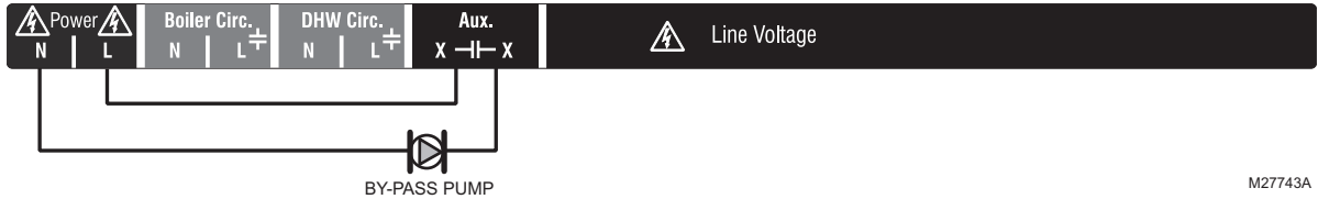
Fig. 16. Wiring of the Aux. pump line voltage rated dry contacts (example shown is a by-pass pump).
