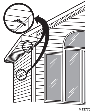
Fig. 7. Outdoor temperature sensor installation.
