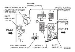
Fig. 4. Top view of ignition system control.
