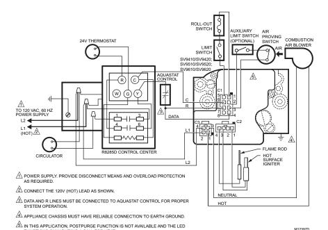
Fig. 9. SV9510/SV9520 typical boiler wiring diagram.
