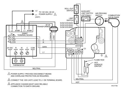
Fig. 8. SV9510/SV9520 typical wiring connection with 208907 Terminal Board.
