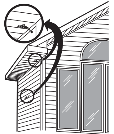
Fig. 7. Outdoor temperature sensor installation.
