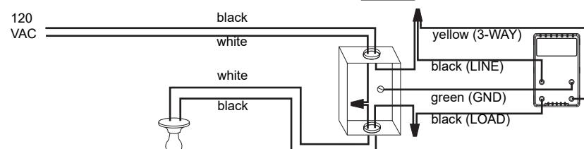
Connect the LINE and 3-WAY wires to the line (120 V) wire and LOAD wire to the load. Connect the GND wire to a ground screw inside the electrical box.
