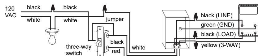
Connect the LOAD wire on the PLS550A/PLS551A to the "common" wire, which you identified when removing the old switch. Connect the GND wire to a ground screw inside the electrical box. Connect the LINE and 3-WAY wires to the two remaining wires. At the other 3-way switch, connect the jumper wire between the "common" screw and the screw where the LINE wire of the PLS550A/PLS551A is connected.
