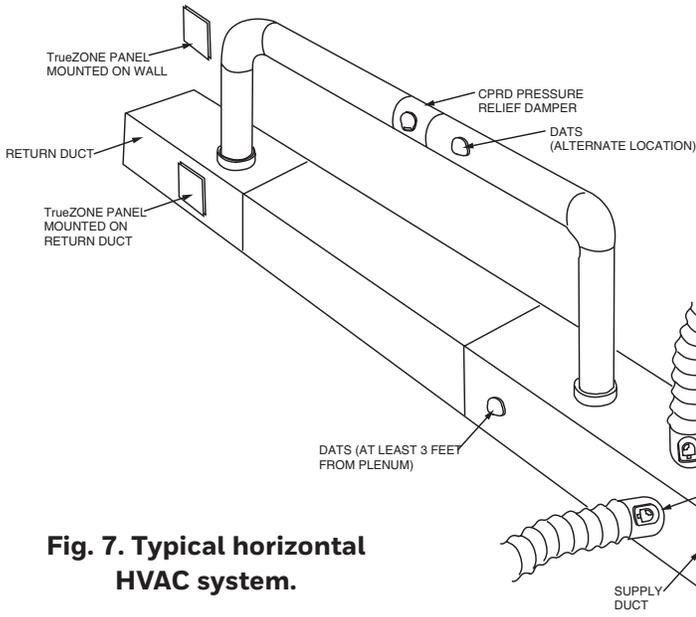
**Fig. 7. Typical horizontal HVAC system.**
