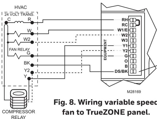
**Fig. 8. Wiring variable speed fan to TrueZONE panel.**
