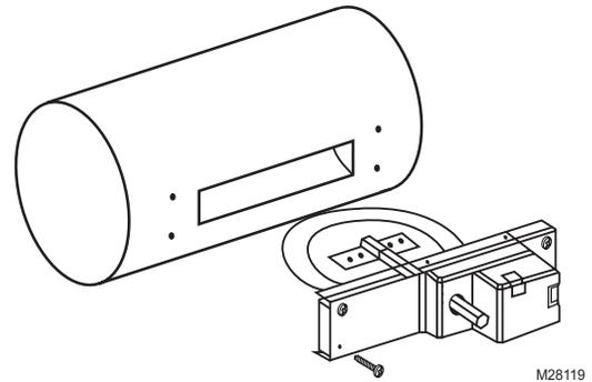
**Fig. 9. Installing retrofit round damper.**
