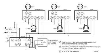
Fig. 5. Wiring L8148E in gas-fired, 24V, forced hot water, no tankless, zoned, pump system.
