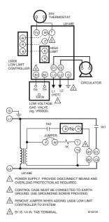
Fig. 4. External connections and internal schematic for L8148E.
