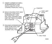
Fig. 11. Adjusting high-limit dial stop with small screwdriver.
