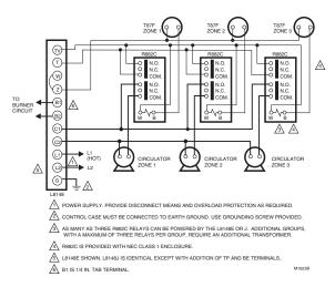
Fig. 10. Multizone system with R882C switched circulator.
