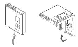
Make the appropriate connections. Please note that the thermostat wires are non-polarized; either wire can be connected to either terminal.
