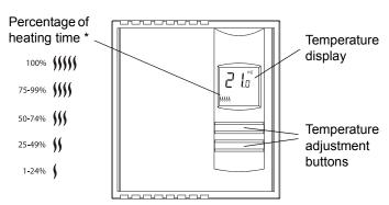
\* The thermostat displays the percentage of heating time required to maintain the desired temperature. For example, 55 is displayed when heating is activated 40 percent of the time.
