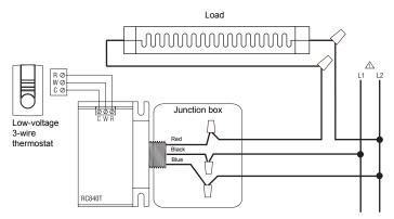
You must provide an overload protection and disconnect as required.
