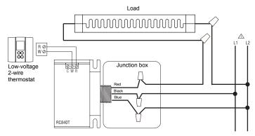
You must provide an overload protection and disconnect as required.
