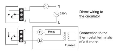
For a 3-wire connection: observe the polarity
