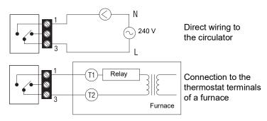
For a 3-wire connection: observe the polarity
