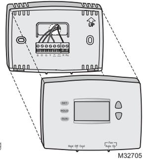
Turn thermostat over, insert fresh AAA alkaline batteries, then reinstall thermostat.
