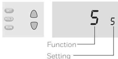
**NOTE:** If you do not press any button for 60 seconds while you are in the setup menu, the thermostat automatically saves any changes made and exits the menu.
