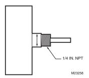
Application: Pressure/temperature gauge with relief set point indicator
