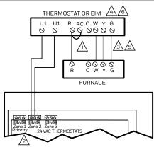
$\stackrel{\frown}{1}$  common wire is optional on most non-wifi models. If cooling is not used, disregard the yand g wires.
