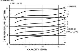
Outlet Pressure Adjustment Range (psi): 0-17 psi Max. Inlet Pressure Rating (psi): 85 Psi Operating Temperature Range: 230°F Maximum (110°C Maximum)
