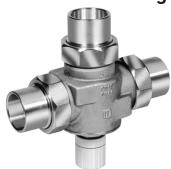
Thermostatic Mixing or Diverting Valves for use in hydronic heating systems as a three-way mixing or diverting valve; controls loop temperature in radiant heating systems.
