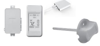
The Prestige® IAQ thermostat is a 2 wire high definition color touch screen thermostat, 7 day programmable and selectable for residential or light commercial use. Controls up to 4-stages of heat and 2-stages of cool in a heat pump system and up to 3-stages of heat and 2-stages of cool in a conventional system.
