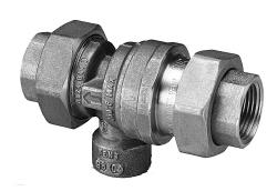
The BP900 backflow preventer is designed for continuous pressure applications on small supply lines. It uses an intermediate vacuum breaker to protect against backflow and back siphonage of contaminated water into portable water supplies.
