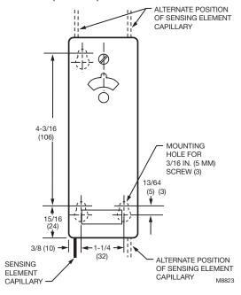
For limiting or regulating temperature of liquids in boilers or tanks. Can also sense duct or outside air temperature.
