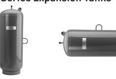
TAX Series (commercial) Expansion Tanks are designed to absorb hot water expansion in closed heating systems of large installations. TAX tanks are equipped with butyl diaphragms to separate the air from the system water (glycol).
