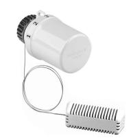
Thermostatic radiator heads are self-actuating controllers which regulate the flow of hot water through thermostatic radiator valves to continuously control the room temperature to the set-point selected on the head.
