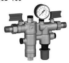
The NK300S Boiler Feed Combination serves as a boiler fill valve used in closed loop heating systems. The NK300S is a (re filling combination valve that contains an integrated pressure reducing valve, strainer, double check backflow preventer with air vent (to protect potable water supply against back flow of heating water into supply pipe), two shut-off ball valves, pressure gauge, and conveniently located test ports for easy inspections and check out.
