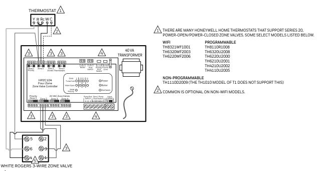
③ THIS DIAGRAM SHOWS THE WIRING ON ZONE 2 BECAUSE IN SOME CASES ZONE 1 IS CONTROLLING DHW. ALL ZONES CONTROLLED BY THERMOSTATS ARE WIRED THE SAME AS ZONE 2 (SHOWN).
