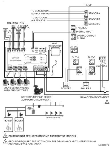
T775P used with Hydronic panels for outdoor reset, and/or staging two boilers.
