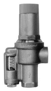
The differential pressure regulator eliminates excessive pump head pressure, when most radiator valves are closed due to reduced demand, by controling flow through a bypass line when the difference between supply/return exceeds the setpoint.
