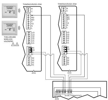
A SEPARATE TH8110R1008 THERMOSTAT AND THM5421R1021 EIM ARE NEEDED FOR EACH WIRELESS ZONE. THE EIMS GET MOUNTED ON A WALL IN THE UTILITY ROOM WITH THE HYDRONIC PANEL. TO ENSURE WIRELESS COMMUNICATING RELIABILITY, WE RECOMMEND THE EIMS BE SPACED AT LEAST TWO FEET APART.
