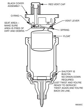
Application: Hydronic heating and cooling Operating Temperature Range: 212°F Maximum (100°C Maximum) Maximum Safe Operating Pressure (psi): 90 psi Maximum Safe Operating Pressure (kPa): 620 kPa **Approximate, Dimensions:** 5 1/4 in. long x 1 7/8 in. diameter (133 mm long x 48 mm diameter)
