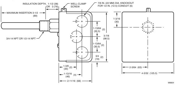
Temperature Range: Maximum – 150°F (66°C) at switches; 265°F (129°C) at sensing element
