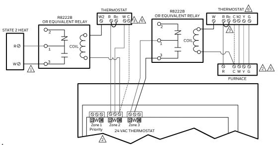
⚠THE WIRING EXAMPLE SHOWN ON ZONE 2 OF THE HYDRONIC PANEL WOULD BE USED IF THE SECOND STAGE HEAT SOURCE DOESN'T HAVE COMMON TERMINAL AND COOLING IS NOT USED. THE WIRING CIRCUIT ALSO ASSUMES THE STAGE 2 HEAT SOURCE HAS A BUILT-IN POWER SUPPLY. IF IT DOES NOT, THE POWER SUPPLY SHOULD BE WIRED IN SERIES WITH THE STAGE 2 HEAT CIRCUIT.
