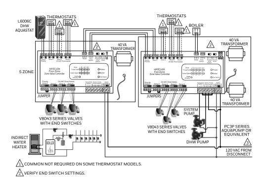
More than 6 zone valves when DHW priority is desired. (DHW is considered one of the zones).
