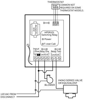
NOTES: GROUND REQUIRED BUT NOT SHOWN FOR DRAWING CLARITY. VERIFY WIRING CONFORMS TO LOCAL CODE.
