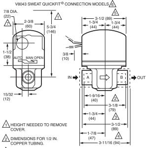
$\stackrel{\textstyle \checkmark}{\cancel{3}}$  DIMENSIONS FOR 3/4 IN COPPER TUBING.
