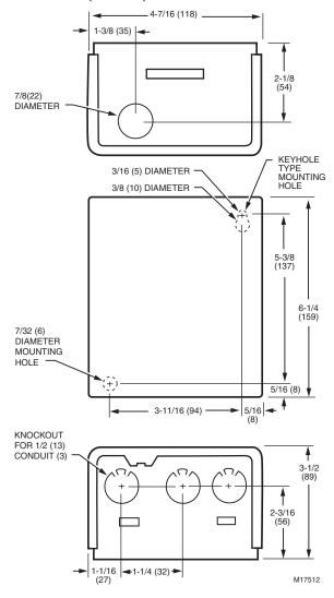
The RA889A Switching Relay with 24 V controller provides intermediate switching of line- and low-voltage devices from a lineor low-voltage controller and is typically applied in Hydronic heating
