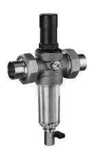
The FK06 DialSet Pressure Regulating Filter Combination is a highquality pressure regulating valve and rinsable filter that maintains a constant outlet pressure over a wide range of inlet supply pressures and ensures a continuous supply of filtered water. It is suitable for potable water and irrigation applications. The downstream pressure adjustment dial eliminates the need for a pressure gauge when adjusting the pressure setting (static pressure only).
