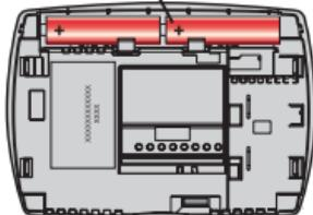
Batteries are optional if your thermostat was wired for AC power when installed. Install fresh batteries immediately when the **REPLACE BATT** warning begins flashing.
