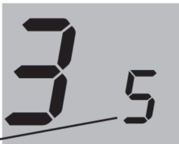
**5** 12 min, Gas or oil furnace. Use this setting if you have a standard gas or oil furnace that is less than 90% efficient.
