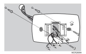
Drill 3/16-in. holes for drywall Drill 7/32-in. holes for plaster
