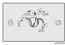
NOTE: Jumper wire used on old thermostat? If yes, note what letters the jumper connected and review in wiring
