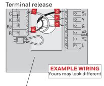
Remove jumper loop ONLY if you have both  ${\bf R}$ and Rc wires.
